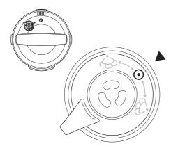
Turn the pressure release valve to the CLOSED position.
