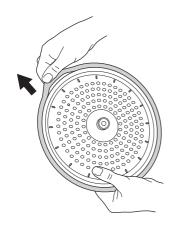
**Removing the gasket:** Pull the rubber gasket from the sides of the inner lid.
