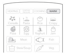
When the timer has finished, your pressure cooker will sound a 'BEEP' and enter the KEEP WARM function, WARM will be highlighted on the display.
