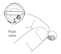
Cleaning the float valve: Clean the float valve using a pin to ensure there is no debris trapped inside or around it.
