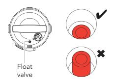
After steam has stopped coming out of the Steam release valve, check that the Float valve has dropped before opening the pressure cookers lid.
