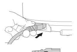
Slot the end of the power cord into the socket on the rear of the pressure cooker as shown in the diagram.
