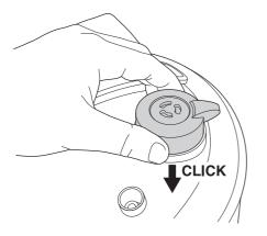
Lower the lid and slot the pressure valve into the large recess on the top of the pressure cookers lid.
