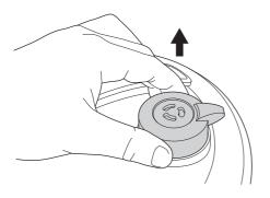
Removing the pressure release valve: Grip the sides of the pressure release valve and pull upwards until it comes off the lid. Use a pin to remove any blockages in the valve.
