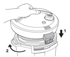
**Refitting the lid:** Slot the hinge on the back of the lid into the channel on the back of the pressure cooker as shown.
